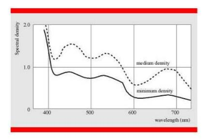
The curves show the spectral density measured on the processed image (neutral object with medium brightness), per wavelength.
