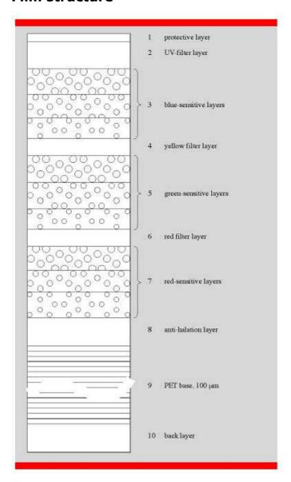
Total film thickness: 100  $\mu$ m PET + 22  $\mu$ m colour layers + 2  $\mu$ m back layer = 124  $\mu$ m.
